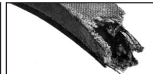
Snub Break Cause: Cover wear indicates slippage and clean break reveals sudden snap due to non-proper drive tensioning. Remedy: Maintain proper drive tension.
