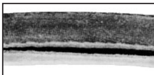
Exposure to Oil & Grease Cause: Belt swelling, exterior softness and bottom envelope seam to open/split. Remedy: Splash Guards, don't over-lubricate, clean belts/sheaves.
