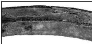
Rough Sheave Sidewalls Cause: Constant slippage due to belt being misaligned on worn sheaves. Remedy: Use correct belt size. Align or replace sheaves.
