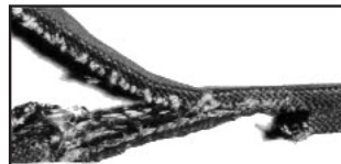
Broken Belt Cause: Rough sheaves and dust build-up can both cause belt failure and severe envelope wear. Remedy: Shield the drive.
