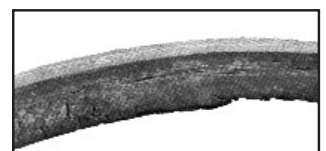
Slip Burn Cause: Belt slipping under starting or stalling load. Remedy: Replace belt and tighten drives until slipping stops.
